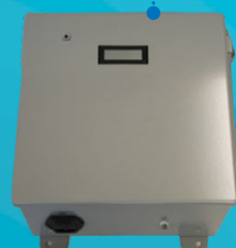
HIGH-FREQUENCY An electronic control unit produces an oscillating radio-frequency electric field that helps minerals drop out of the solution.
